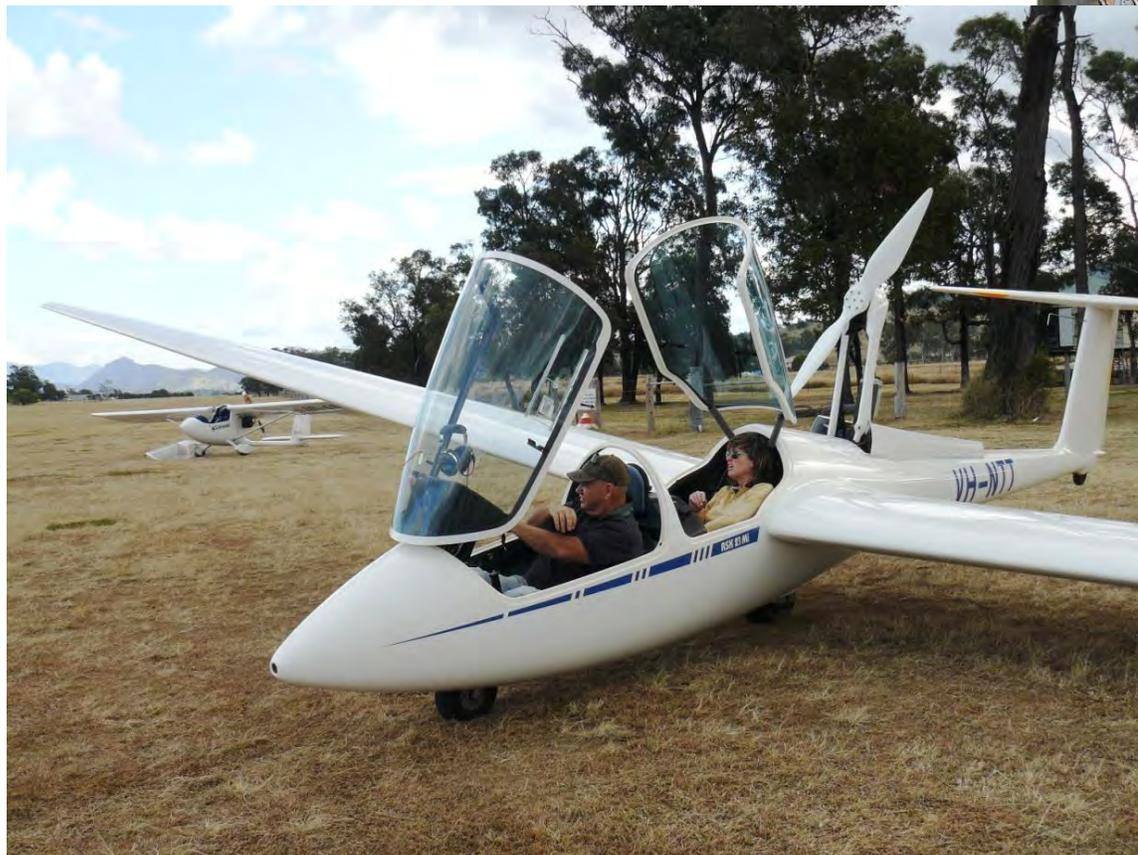
struts or springs (not sure which). The instrument panel for the front cockpit is actually attached to the front canopy (see photo above). The photo on the left shows a happy couple about to taxi out onto R22 for a pleasant jaunt over Boonah and surrounds. All things considered, I felt there was only one small problem with the ASK21 and that was the cost – about five times as much as that other little “motor glider” in the background.
