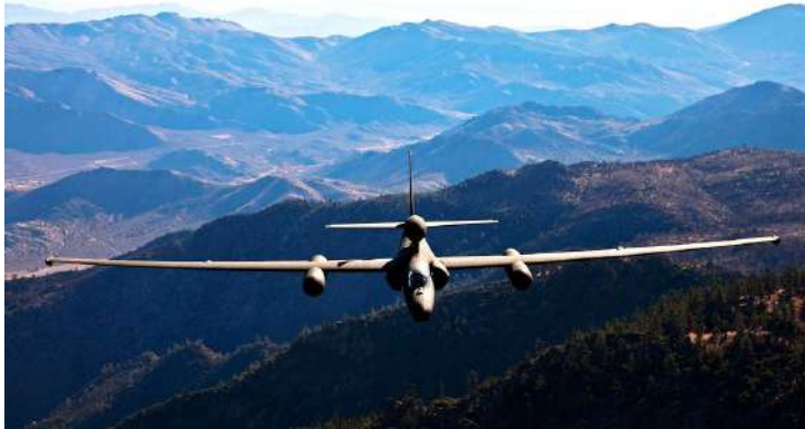
The U-2's design - a slim body and long wings - help keep it aloft in the thin air of the upper atmosphere (Credit: Lockheed Martin)
