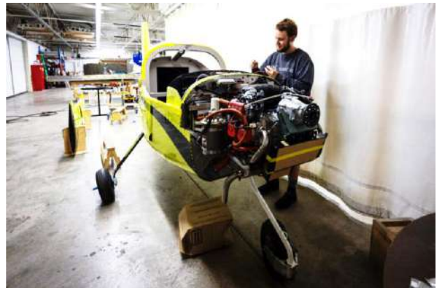
The process for putting together the Van's-built light sport RV-12 follows the same path, essentially, as an owner would when building the ELSA version from a kit—except technicians build a couple each month rather than one in a lifetime. [Credit: Stephen Yeates]
