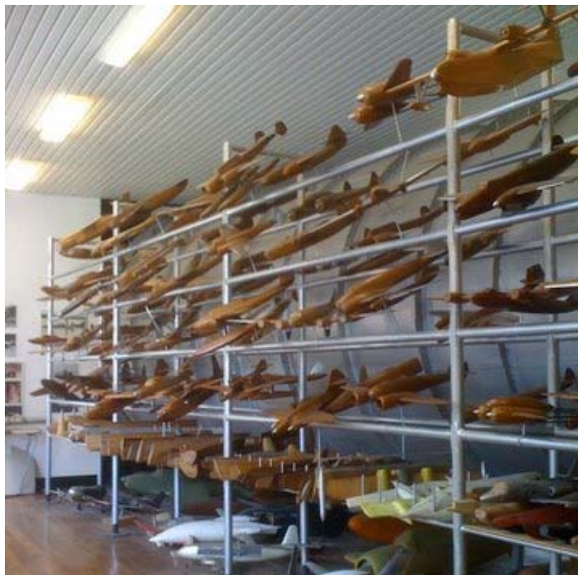
Above: Impressive collection of carved mahogany aircraft models used in the wind-tunnel, dating back many decades. Photo by Mark Bolsover.
